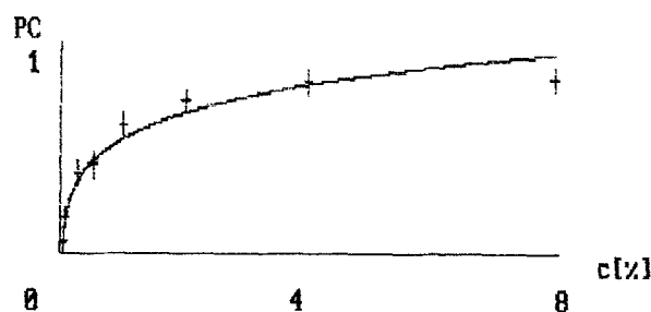
Figure 16. Perturbation coefficient PC = 1 - |\vartheta| of yeast vs formaldehyde concentration c . Direct proportionality between the perturber concentration and its effect is maintained using this definition. However, the range of application of the definition is limited to the cases when a reference process is stationary and uncorrelated (see input process \{a(t)\} in fig. 14).
